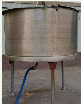
Smaller calf milk vat (left). Some farms store water here for peak season chilling, if large enough. Calf vats do not need wrapping.
